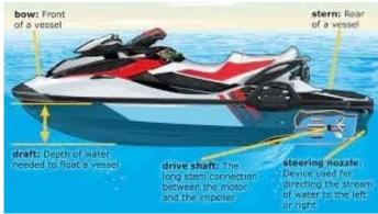
Jet intake area, located near the drive shaft and steering nozzle, sucks in water and then passes water through a high-speed impeller. This will make the steering nozzle thrust the jet-ski forward.
