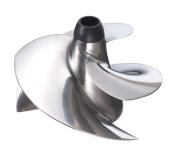
Jet-skies use impellers, like the one seen to the left. The impeller is the primary driver of the jet-ski, as the three blades force the water pumped in, out at a much higher speed in the opposite direction of motion. The impeller is within a pipe that runs from the water intake to the nozzle at the rear. They spin very rapidly so it is important to keep the impeller clear at all times and clean it out if anything gets caught inside. Make sure to do this with the engine off.
